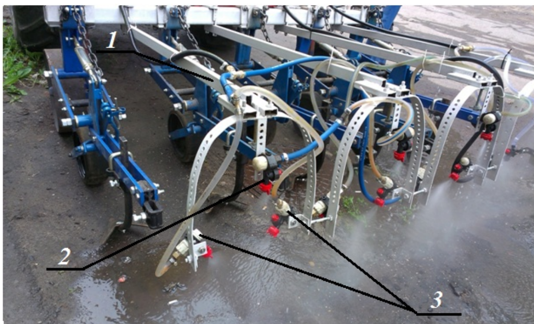
1 - cultivator; 2 - upper sprayer; 3 - side sprayers;
