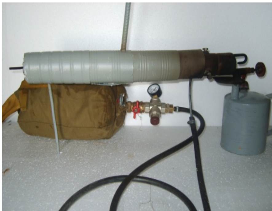
Figure 1. Scheme of autonomous steam generating installation: 1– torches, 2– crane, 3 – built-in pump., 4 – casings, 5 – account capacity, 6 – fastening, 7 – capacity for water, 8 – gate, a 9 – copper tube, 10 – the handle
