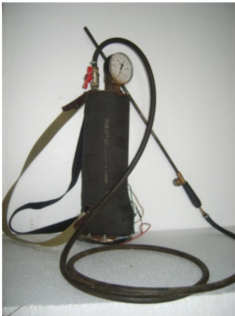
Figure 2. Electric steam generating installation: 1 – account capacity, 2 – jellied mouth, 3 – heating element, 4, 5 – the main and waste valves, the 6 – emergency automatic device, 7 – bar, the 8th nozzle, the 9– regulating crane, 10– generator
