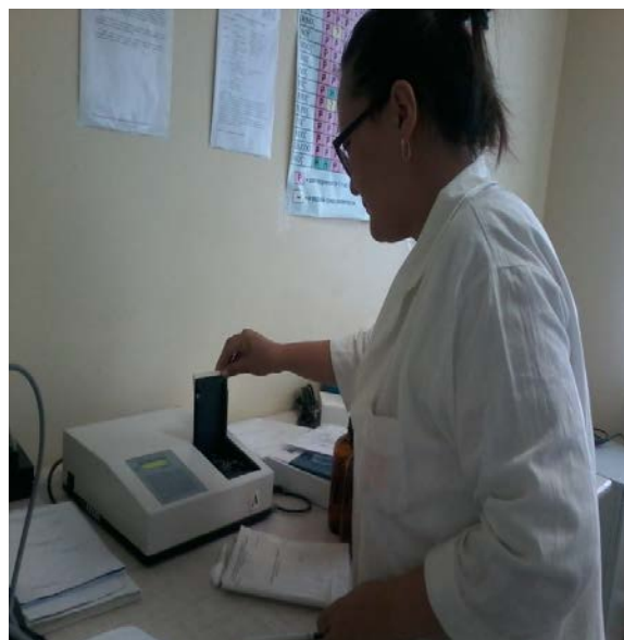
Figure 1. Determination of phenols and oil products to the fluorometric analyzer fluid "Fluorat-02-3M"
